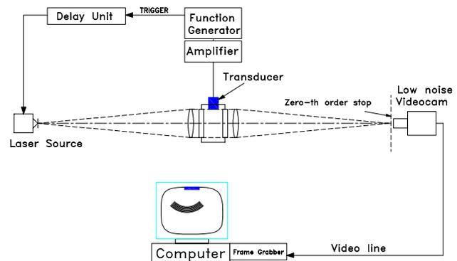
**Figure 1.** Diagram of the quantitative schlieren system used.
