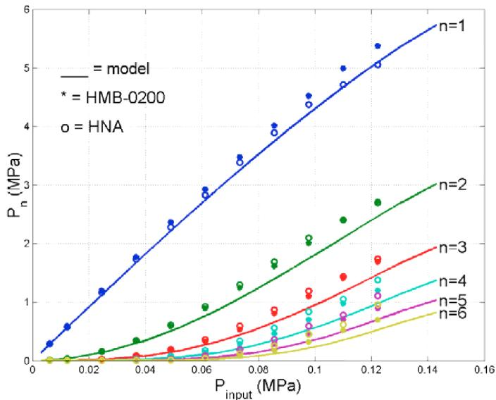
**FIGURE 6.** Amplitude of harmonic content of pressure waveforms as a function of average pressure across the face of the source transducer.  $n = 1$  is the fundamental (1.505 MHz),  $n = 2$  is 3.01 MHz, etc.
