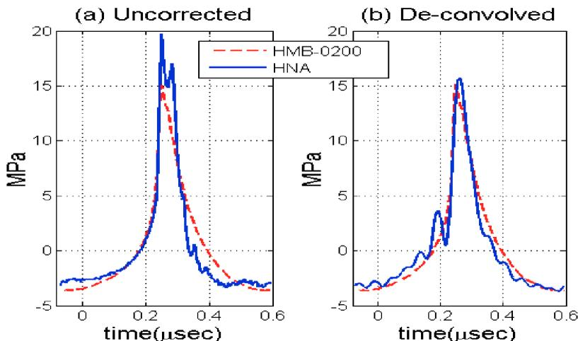
**FIGURE 4.** Single cycle of pressure waveform at focus. (a): HNA and HMB-0200 voltage waveforms scaled by their respective sensitivities at 1.505 MHz. (b): Data corrected by amplitude deconvolution using the calibration data shown in Fig. 3.
