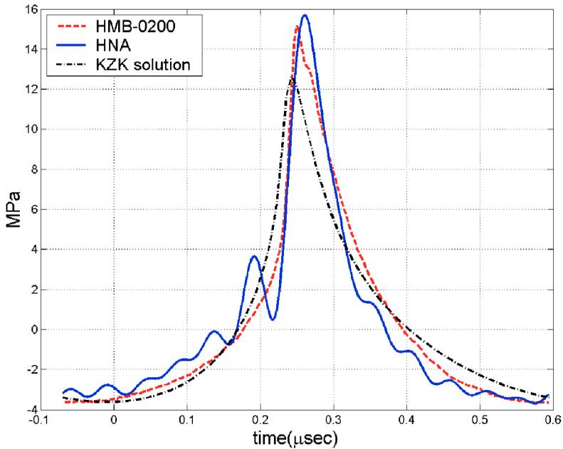
**FIGURE 5.** Single cycle of pressure waveform at focus. The HNA and HMB data are corrected using the sensitivity amplitude data, as in Fig. 4 (b).
