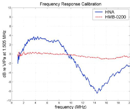
**FIGURE 3.** Sensitivity calibration of the HNA and HMB hydrophones used in this study, normalized by their respective sensitivities at driving frequency (147.9 mV/MPa for the HMB, and 56.6 mV/MPa for the HNA).
