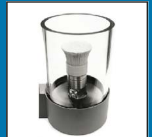
Brush target for HIFU measurements Up to 100W (RFB-BTK)
